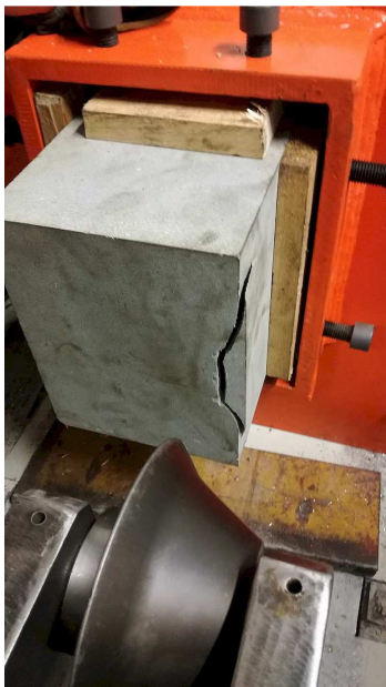
Fig.9. A view of the sandstone block after the mining test ( R_c = 79 MPa) - disc \varnothing 150/40^\circ , t = 15 mm
