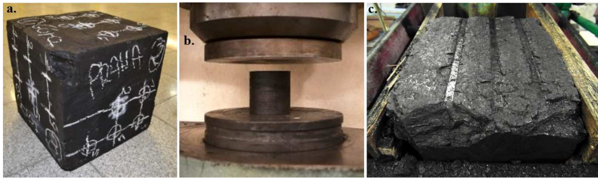
Fig. 3. The investigation into hard coal: a. provided sample b. before R_c tests, c. after cuttability index tests
