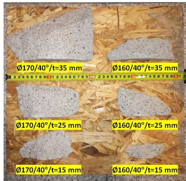
Fig.10. Graining of the output obtained during the mining tests with single disc tool ( R_c=25 MPa)
