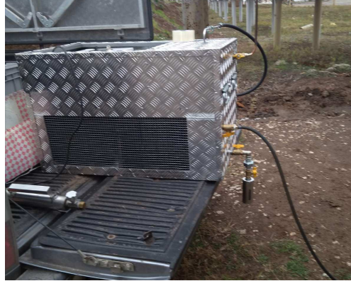
Fig. 1. Laboratory unit for OAG separation “LURPNG. Source: Self-elaboration.
