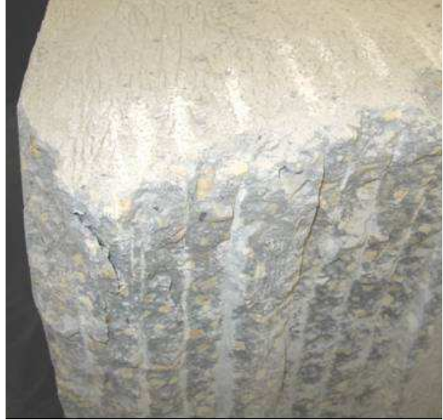
Fig.12. A view of the concrete block surface after completing the mining test
