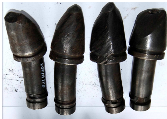
Fig 1. Examples of conical picks used in the cutting drum of a roadheader withdrawn from operation
