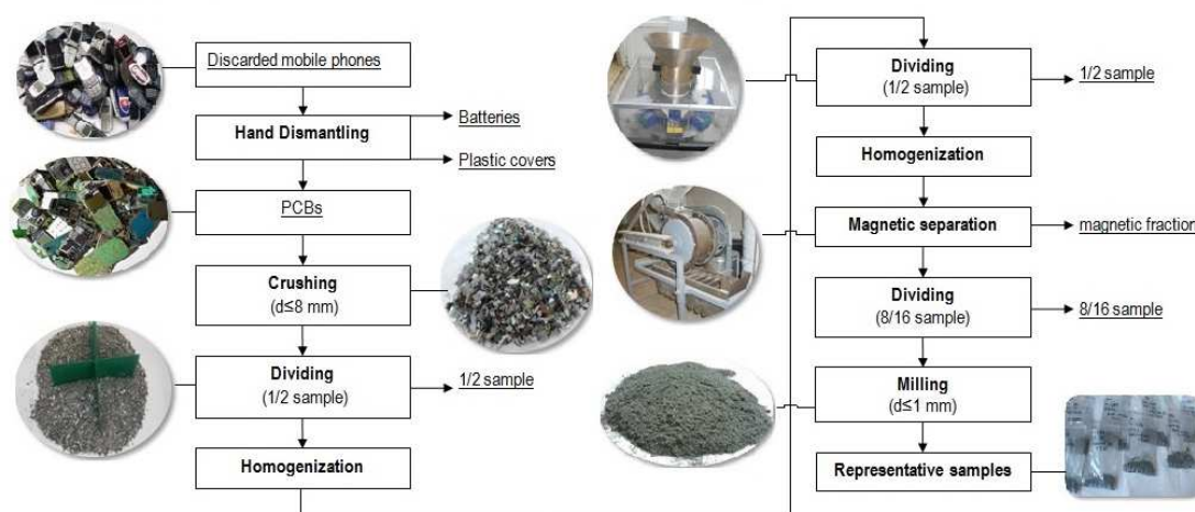
Fig. 1. Methodology for printed circuit boards sampling from discarded mobile phones
