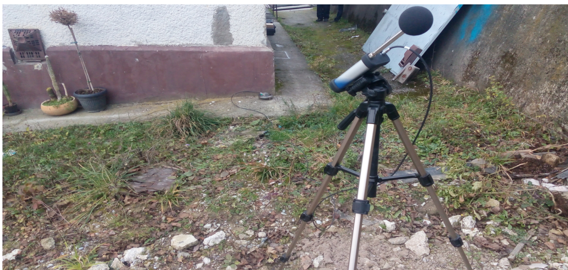
Fig. 8. SVAN 958A installed near a residential building in Nimnica (Fehér et al., 2019)
