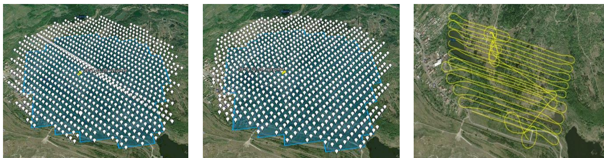
Fig. 4. Flight line trajectories (from left eBee 1 (left), eBee 2 (middle) and Easystar (right)).
