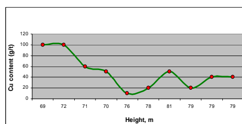
Fig. 26. Distribution of Cu along the edge of No. 1 Open Pit depending on the relief
