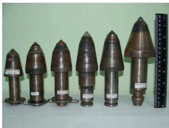
Fig. 2. Model range of cutters for various combines.
