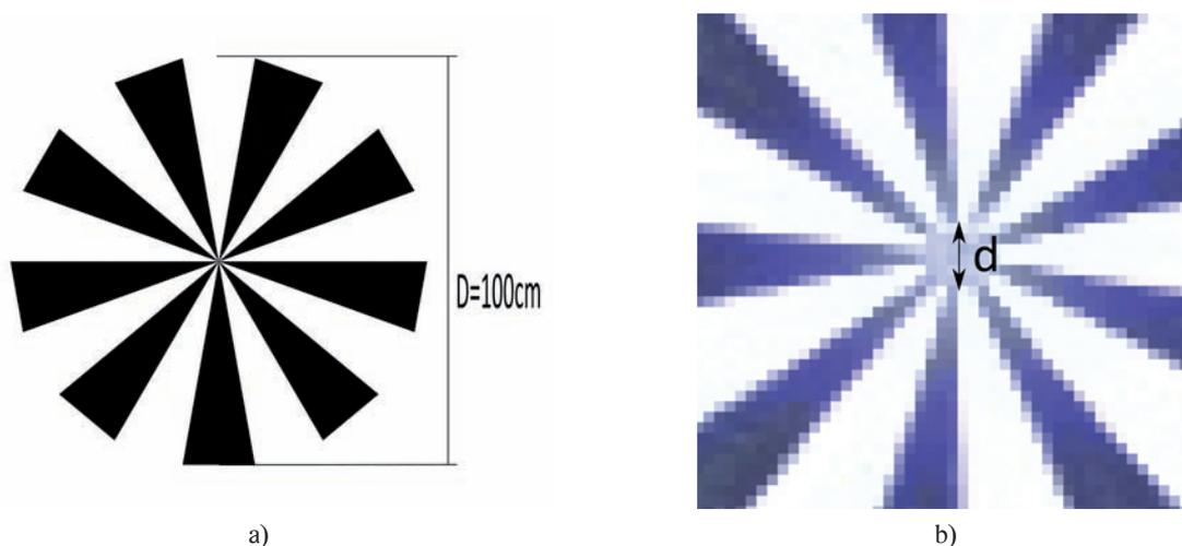
Fig. 1. Siemens star calibration target used in study (a). Blurred center (with diameter  $d$ ) of Siemens star calibration target (b).
