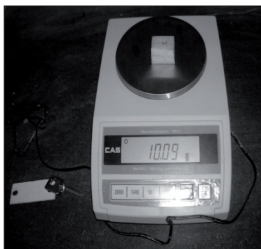
Fig. 6. Electronic laboratory scale MWII-200B.
