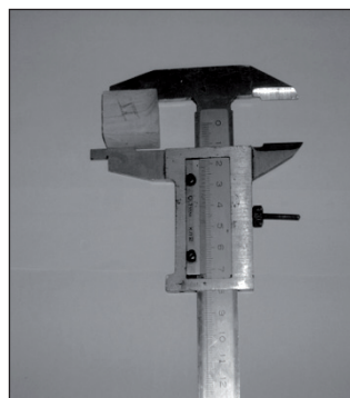
Fig. 7. A calliper, accuracy class 2.
