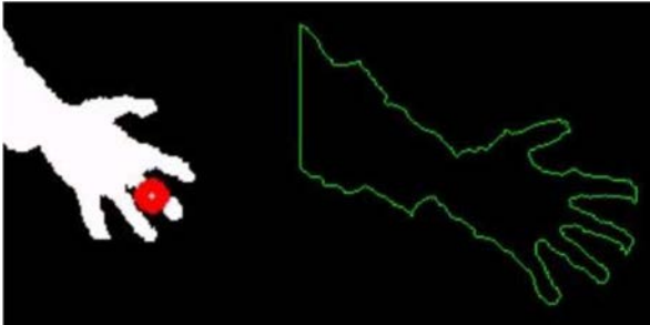
Figure 6 ROI around the right palm and corresponding contours detected by Suzuki85 algorithm.
