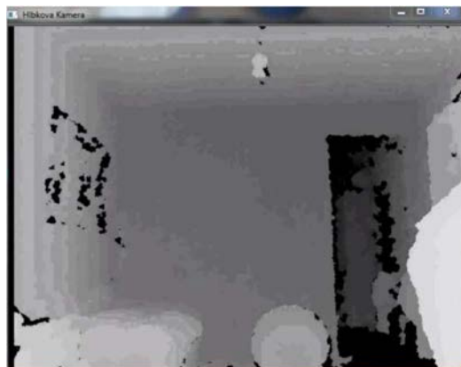
Figure 4 Disparity map obtained from Microsoft Kinect. Black dots represent incorrect measurements. This is due to objects situated closer than minimal measuring range or visible light, which transilluminates the transmitter.
