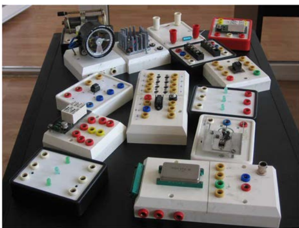
Figure 1 Several parts of building items for prototyping of mechatronic systems
