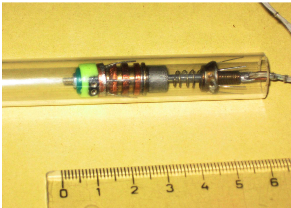
Figure 1 Machine with electromagnetic actuator
