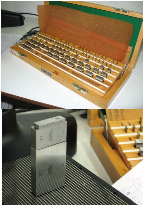
Figure 6 Set of length gauge blocks and building of length etalons
