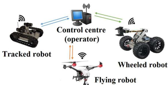
*Figure 1 Scheme of control of different kind robots*
