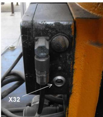
Figure 11 Connection cable for EMT
