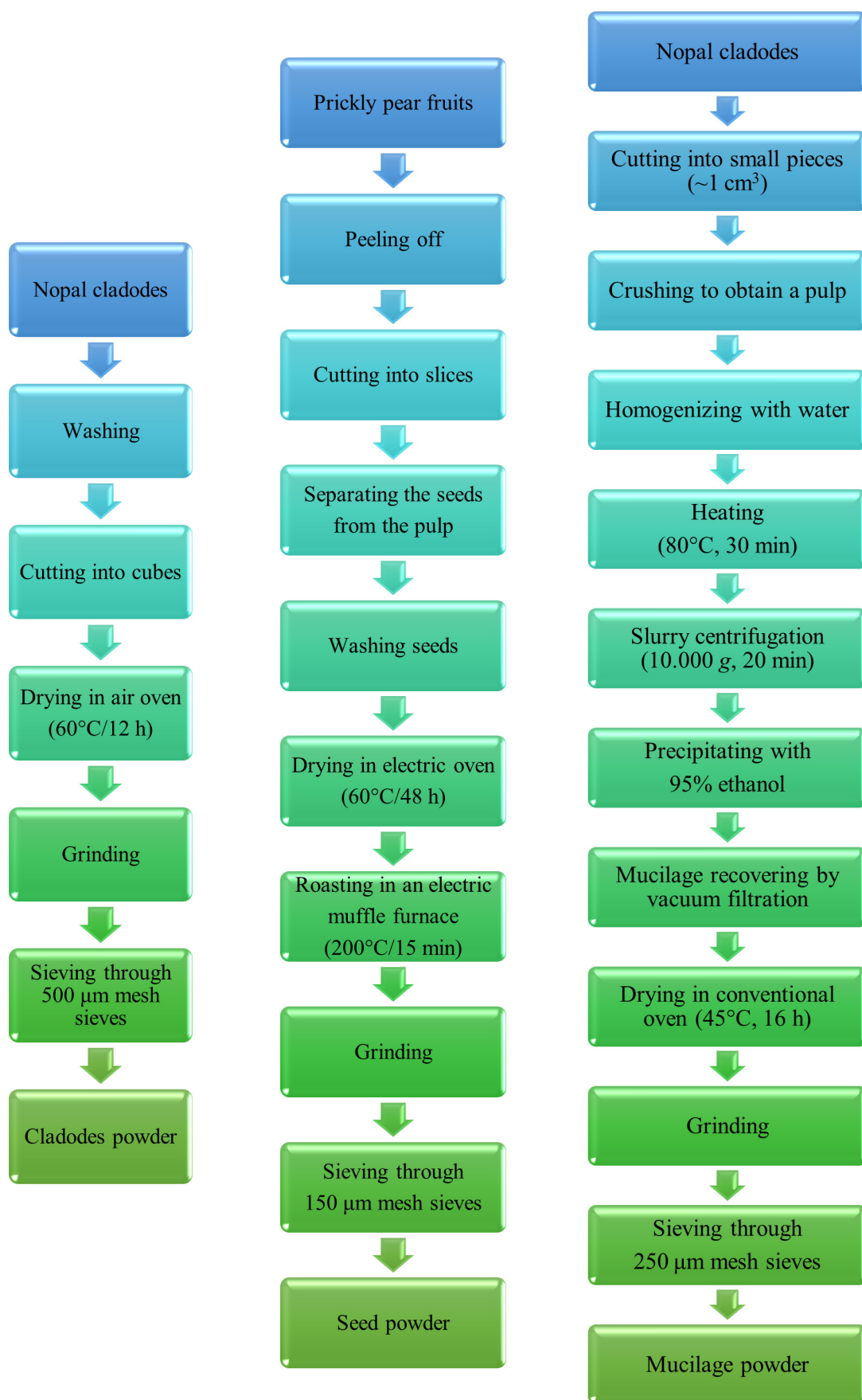
Fig. 1. Flow chart of processing different parts of Opuntia ficus-indica into cladodes, seeds and mucilage powders (Contreras-Padilla et al., 2016; Dick et al., 2019; Reda and Atsbha, 2019; Ali et al., 2020; Dick et al., 2020; Nabil et al., 2020; Chaloulos et al., 2021; Sciacca et al., 2021).
