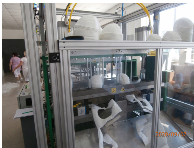
Fig. 2. Automated extrusion line for nanotextile respirators.
