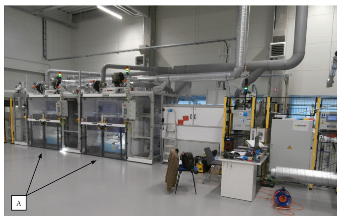
Fig. 1. Large-capacity production line for continuous production of nanofiber textiles at Nano Medical s.r.o. Letter A indicates the location of the spinning units with containers of polymeric material.
