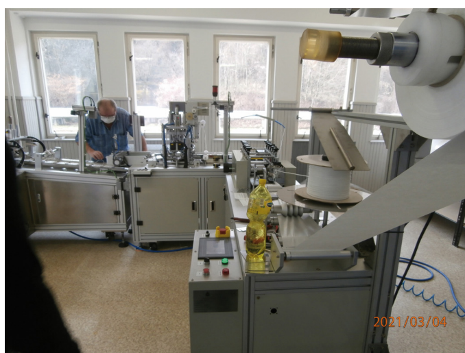
Fig. 3. Automated line for nanofiber masks Nanovia Mask 99,97 production.
