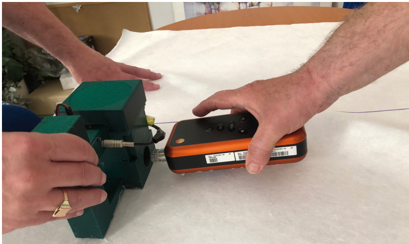
Fig. 5. Experimental equipment for blowing fibers (nanofibers).
