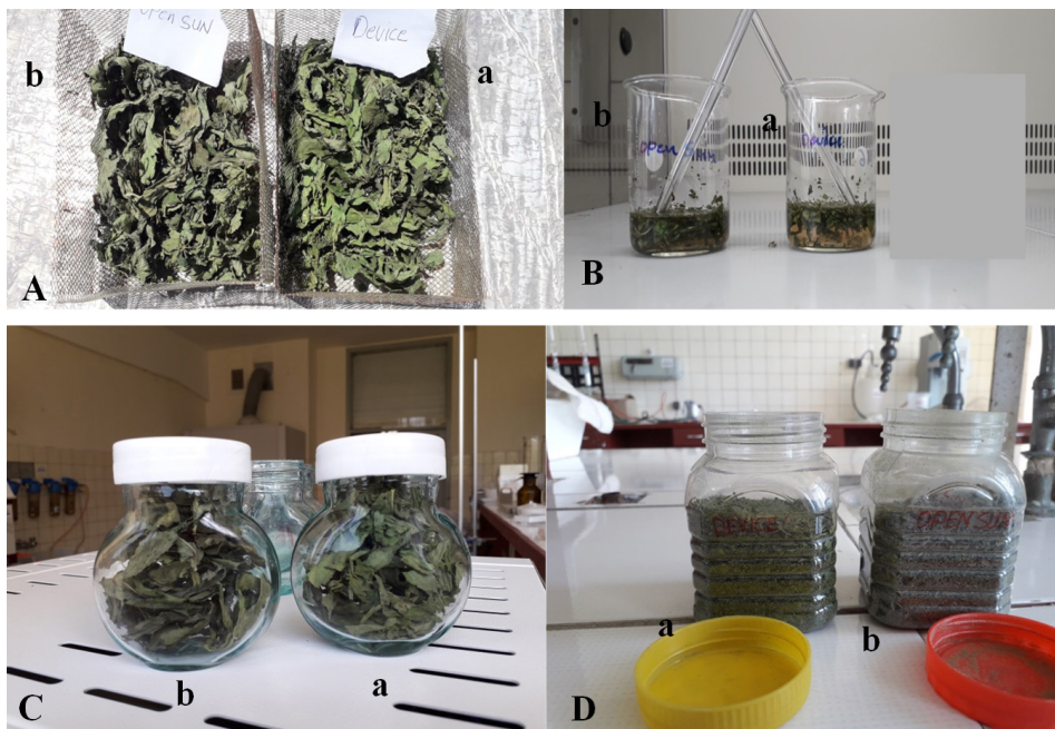
Fig. 12. OSD and AISD product color comparison: a – AISD products, b – OSD products.
