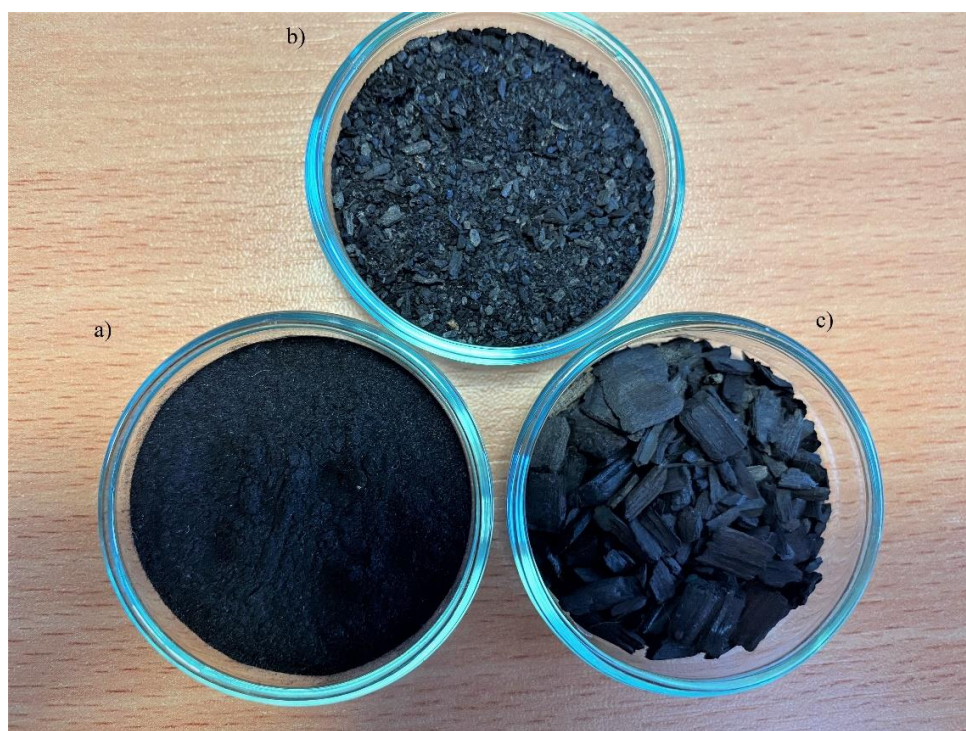
Fig. 1. Biochar fraction sizes a) <125µm, b) 125µm–2mm and c) >2mm.
