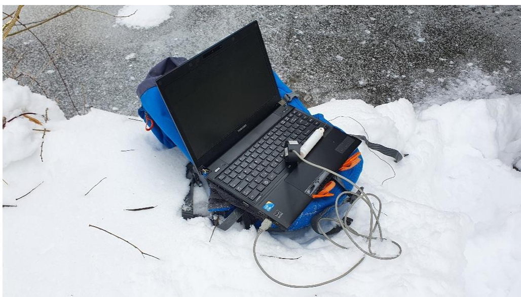
Fig. 3. Equipment for downloading water temperature data (portable field computer, Minikin Tie temperature sensor and IrDA cable).
