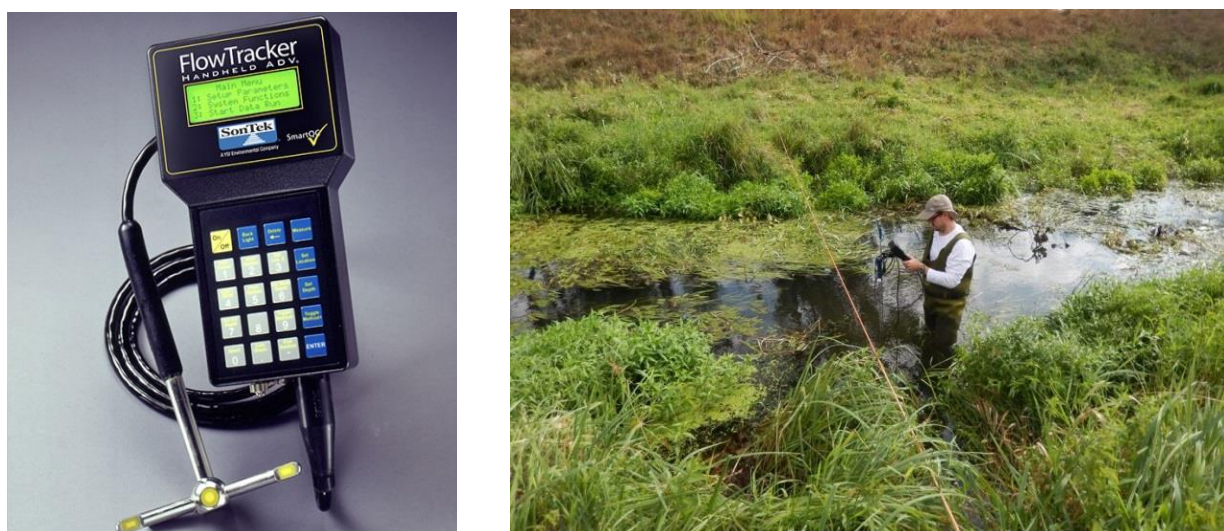
Fig. 2. Acoustic Doppler Velocimeter – Flow Tracker device for measurement of velocity profile and discharge (left) and photo of the overgrowth of the Malina stream during summer season (right).
