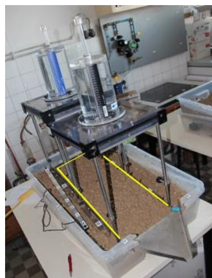
Fig. 1. The Eijkelkamp rainfall simulator: A – sprinkler plate and water reservoir, B – adjustable support, C – ground frame, D – small capillaries, E – adjustable support, F – aeration pipe.
