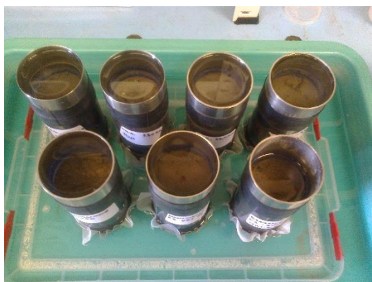
Fig. 3b. The demonstration of application of falling head method to 24 undisturbed samples from Chotárny channel.
