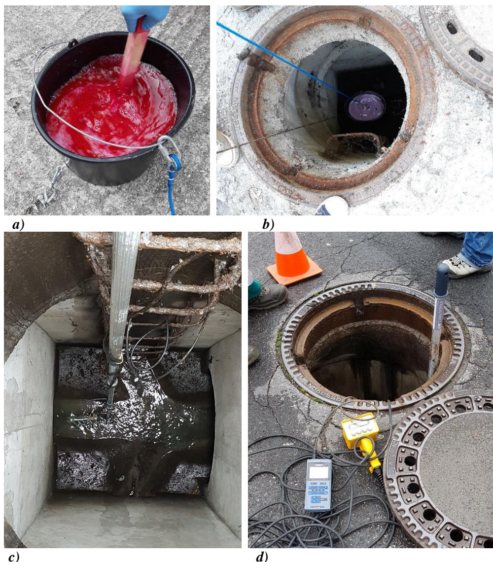
Fig. 1. Documentation of the experiment steps: a) tracer preparation, b) tracer dosing, c) measuring probes in the confluence manhole, d) data loggers for recording the measured data.
