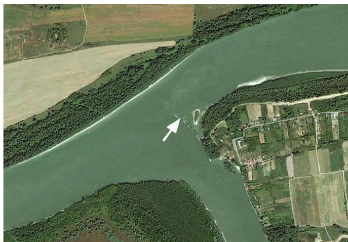
Fig. 8. The directing flow dam (shown by the arrow) at the division of the Danube River into Kiliyskyi and Tulchynskyi branches.
