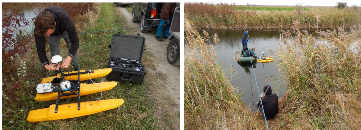
Fig. 4. Equipment for measurement of the velocity profiles and discharges in the channel – RiverSurveyor S5/M9.
