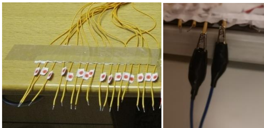
Fig. 6. Switching between individual sensors.
