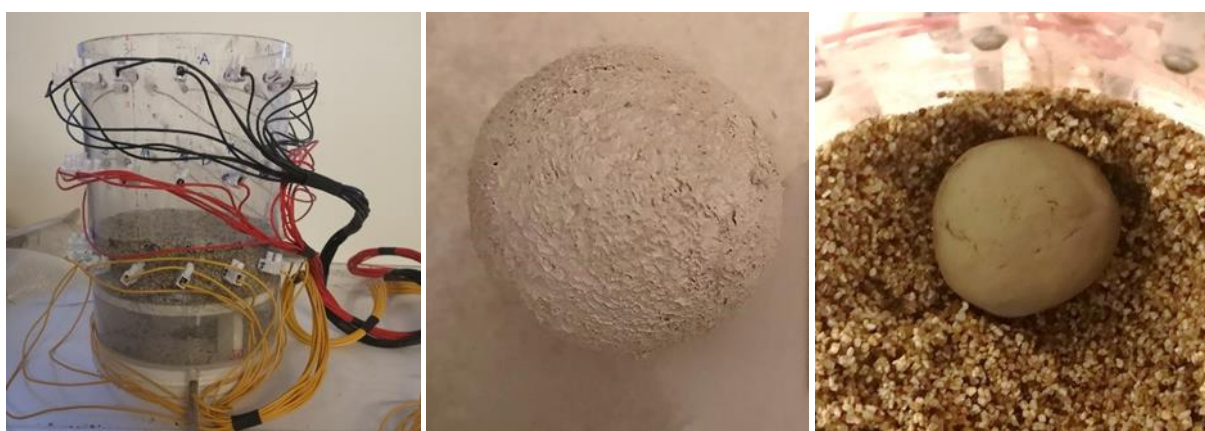
Fig. 7. A model with a sample of sand – left, a sample of clay – in the middle, sample of clay inside the environment – right.
