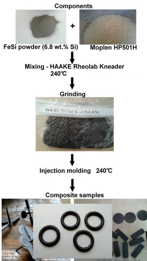
Fig. 2. Preparation procedure of the FeSi-polypropylene composite samples, using injection molding
