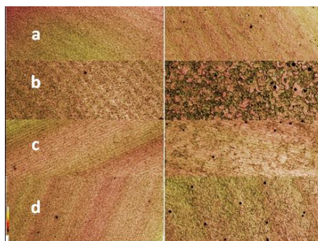
Fig. 4b. Confocal microscopy figures of WC coatings deposited on WC-Co (left)
