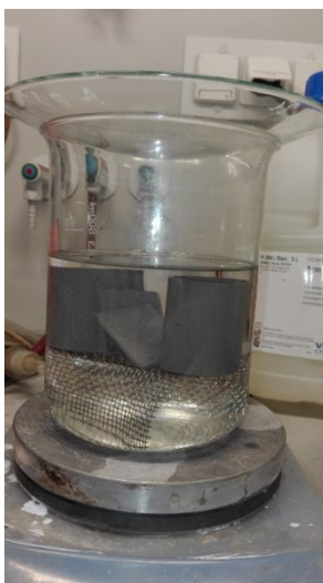
Fig.4. Beaker filled with cyclohexane for debinding.
