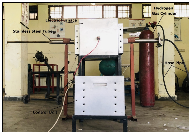
Fig.1. External view of sintering machine.
