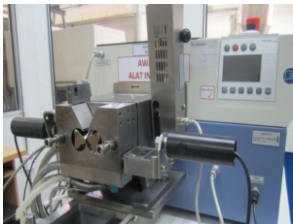
Fig.1. Twin-screw Brabender mixer W50 EHT.
