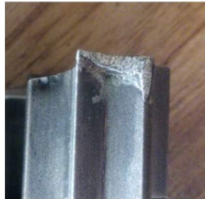
Fig.6. Repaired area before machining.
