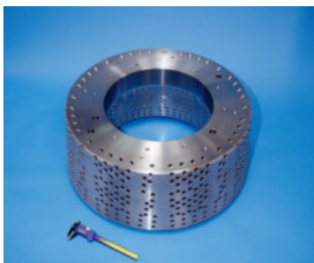
Fig.5a Heavy alloy collimator for radiotherapy (mass approx. 2 tons)(Plansee SE).
