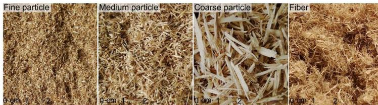
Fig. 1: Wood particle and fiber used for manufacturing of low density particleboard.
