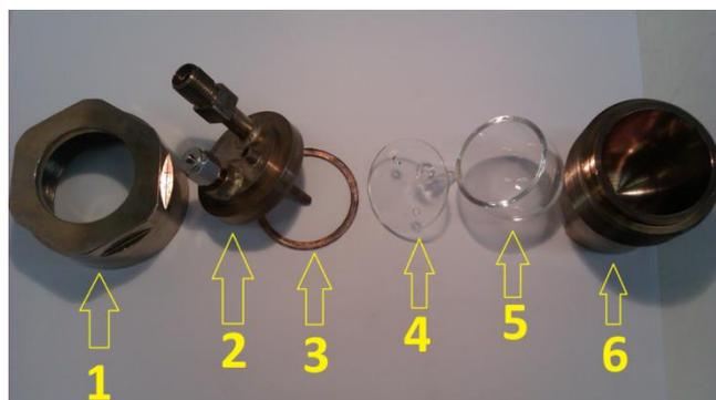
**Figure 1 SEDEX stainless steel vessel assembly 1: Top part 2: Lid 3: Copper o-ring 4: Glass liner top 5: Glass liner bottom 6: Bottom part**
