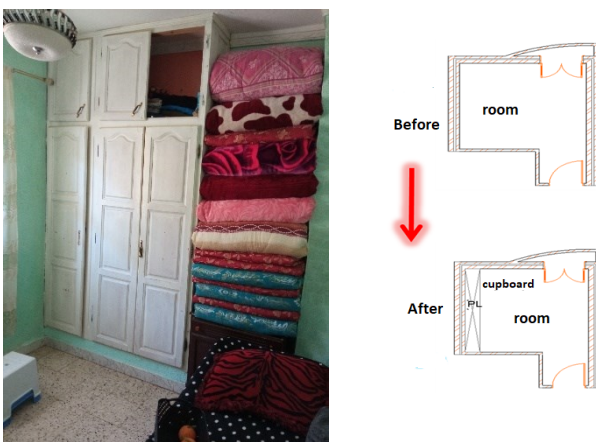
Fig. 15. Installing a cupboard. (Source: Authors, 2023)
