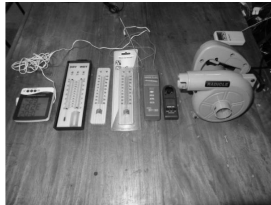
Figure 5 Photographic view of data measuring instruments: (a) Data logger (b) Digital thermometer, hygrometer, anemometer, and blower.
