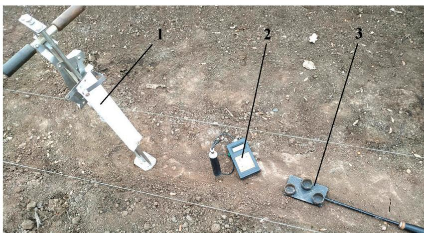
**Fig. 3** Devices for determination of physical and mechanical properties of the soil in tracks of permanent traffic lanes
