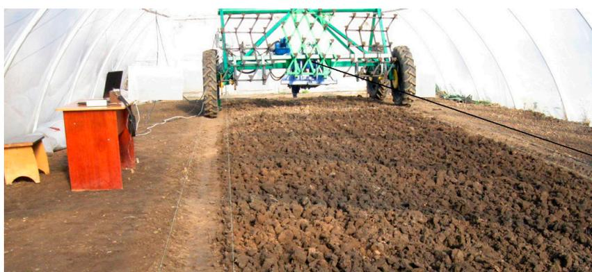
**Fig. 1** Experimental agricultural bridge equipment during a laboratory research of its rolling resistance along the permanent traffic lanes
