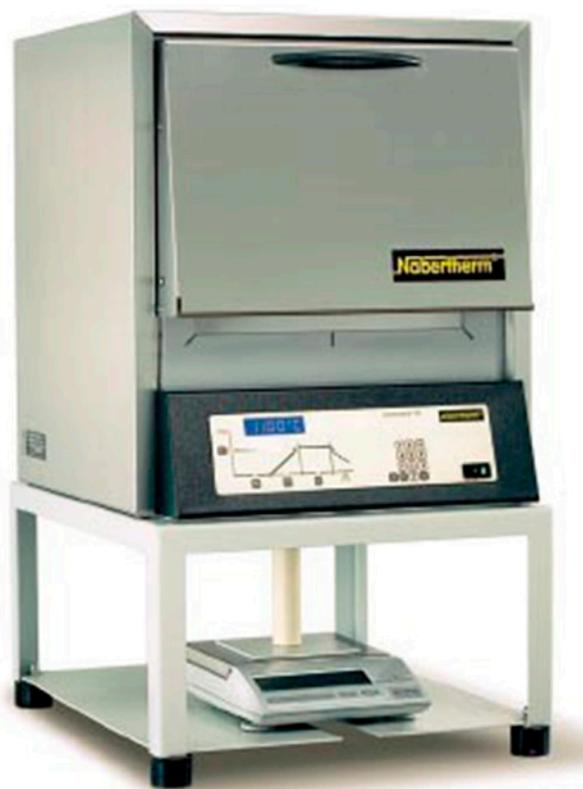
**Fig. 1** Apparatus for thermogravimetric experiments
