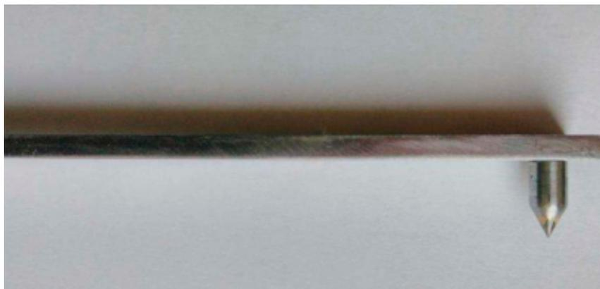
**Fig. 2** Diamond tipped gauge used for surface roughness measurement
