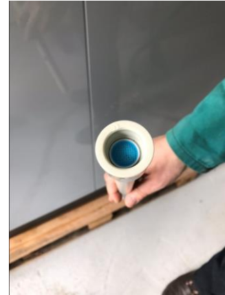
Figure 9 Inserting the strainer into the measuring element
