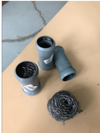
Figure 6 Inserting the wires into the measuring element
