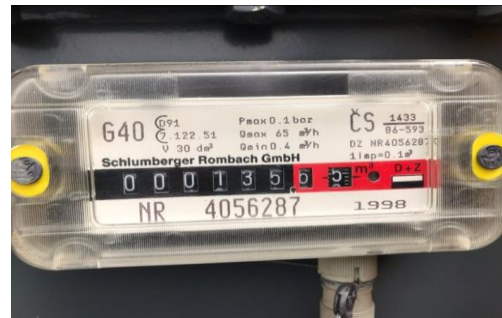
Figure 4 G40 BK volumetric flowmeter used in natural gas measurement
