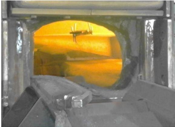
Figure 4 View of a sample and rack applied to a billet placed in a heating furnace
