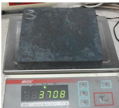
Figure 6 View of a sample after complete descaling subjected to weighing
