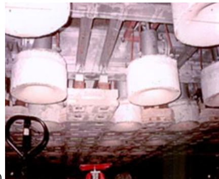
Figure 5 The roof of the reheating furnace made from prefabrications [6]
