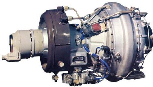
Figure 8 The AI-9V air generator
