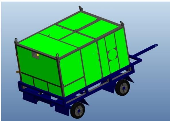
Figure 9 The design container placed on a wheeled chassis [8]
