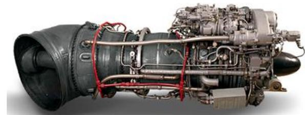
Figure 4 View of the aviation turboshaft helicopter engines TV3-117 [5]
