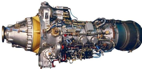
Figure 1 Turbo propeller engine AI-24VT [5]
