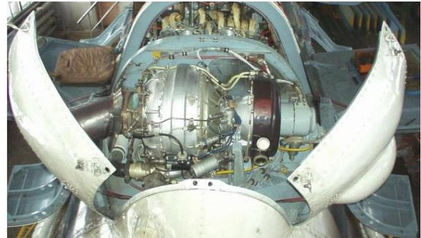
Figure 6 Location of the air generator on the Mi-24 helicopter [8]
